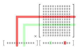
A typical  $\mathbb{F}_2$  vector-matrix multiplication implementation loops over the vector and accumulates matrix lines with XOR if the element is set.
