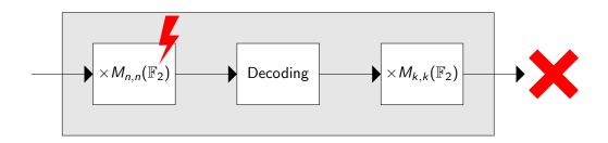
Making a fault-injection based attack work on McEliece is hard because attempts :
